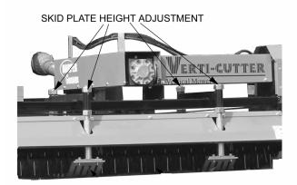
The skid plate height determines the cutting depth of the blades.
