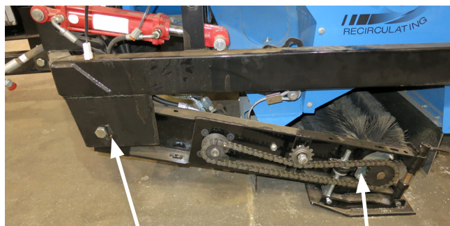
Deck Hinge Shaft
