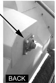
ZERKS ON BLOWER SHAFT
