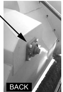
ZERKS ON BLOWER SHAFT
