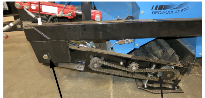
Deck Hinge Shaft
