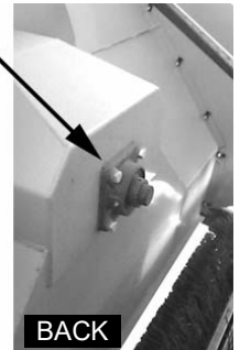
ZERKS ON BLOWER SHAFT
