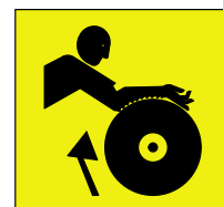
9. Contacting moving parts will cause injury
