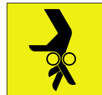
8. Hand can be entangled in moving parts
