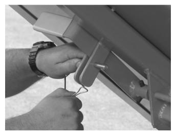
To engage the cylinder safety lock, take the pin out of the bracket on the hopper and pull the handle down.
