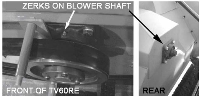
**Note:** The safety shield must be removed to access grease zerk on front blower shaft of the **TV60RE**.
