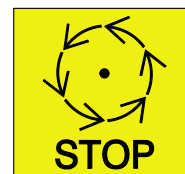
10. Turn off equipment before performing maintenance
