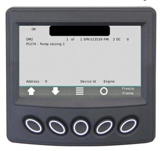
**NOTE:** Select the Freeze Frame Button to requests the freeze frame data from the ECU when faults are present.
