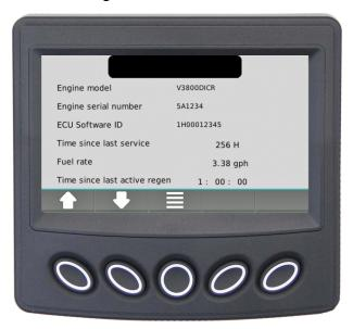
Press the UP/DOWN soft keys to display a screen with application and configuration information.
