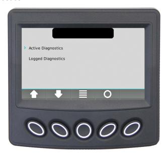
Active Diagnostics: Use the UP/DOWN soft keys and stop the cursor (...) next to the action item Active Diagnostics. Press the select ( ) soft key .The screen displays active warnings or faults from the ECU. Each diagnostic is shown with the appropriate Suspect Parameter Number (SPN) and Failure Mode Indicator (FMI), Text Description (if available), and the ID/Name of the device that transmitted the DM1 message. Press the UP/DOWN soft keys to reach the next diagnostic in the list.
