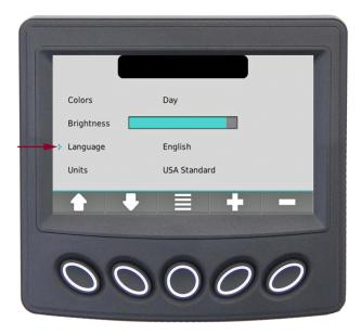
**Units:** Use the UP/DOWN soft keys and stop the cursor (...) next to the action item **Units.** Set your unit preference using the +/– soft keys.
