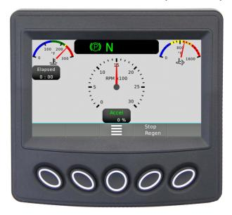
Parked Regeneration is complete when the controller screen shows the following green popup message. Click on the soft key to remove the popup message. The machine can return to normal usage.
