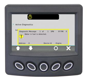
**Logged Diagnostics**: Use the UP/DOWN soft keys and stop the cursor (...) next to the action item **Logged Diagnostics**. Press the select ( ) soft key. The screen displays the controller requests DM2 (stored trouble codes, not active), warning or faults from the ECU. Each diagnostic is shown with the appropriate information:
