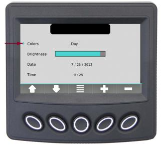
**Screen Brightness:** Use the UP/DOWN soft keys and stop the cursor (...) next to the action item **Brightness.** Set the brightness of the backlight by using the +/– soft keys.
