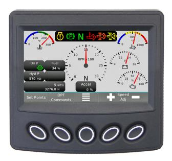
The gauge screen displays five (5) dial gauges and as many as seven (7) digital gauge options.
