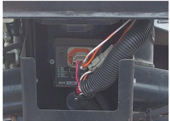
**Inclinometer Module** – senses if the machine is off center/vertical. The machine can lean to either side up to 34° before reaching its limit.
