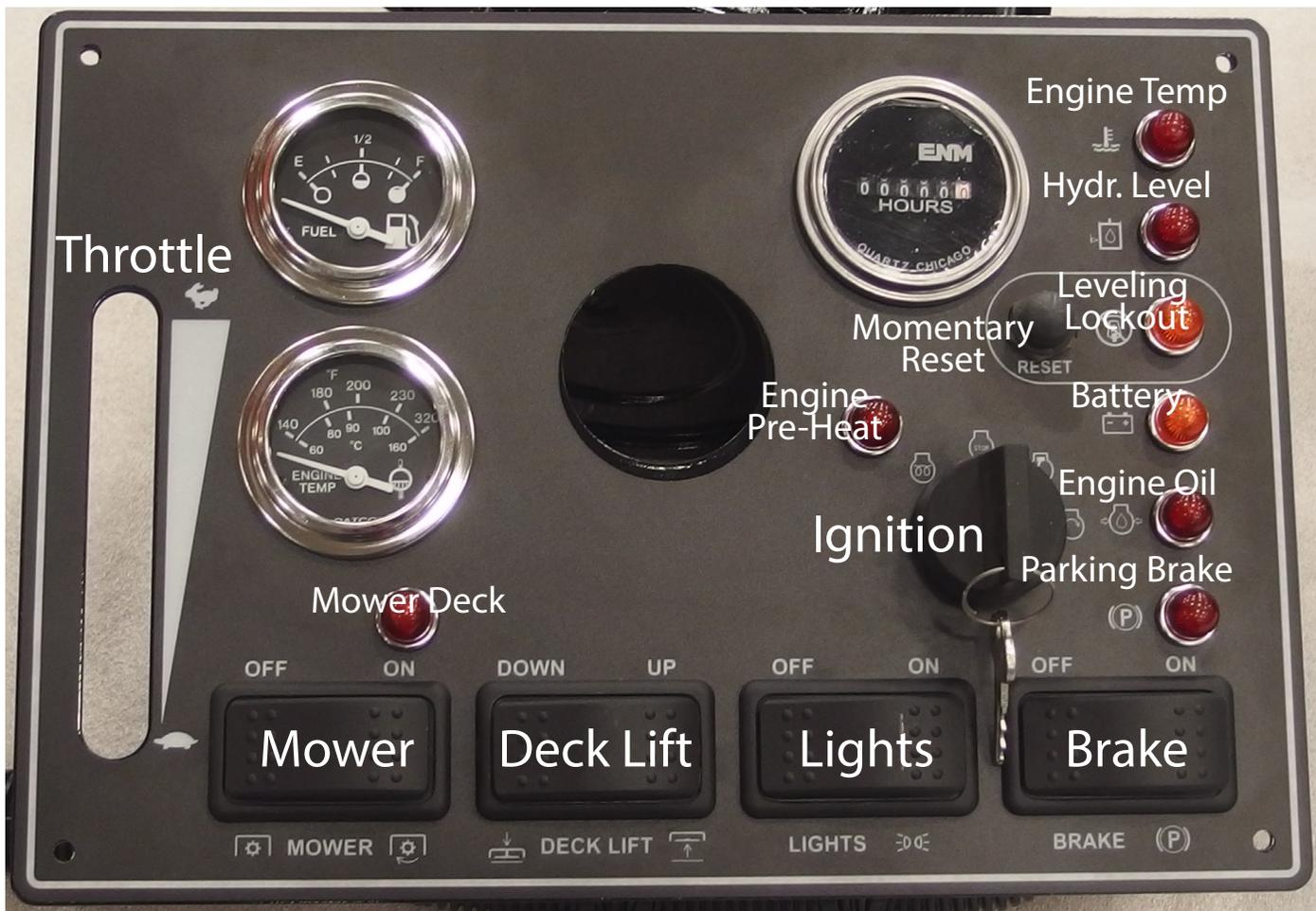
**Throttle** – adjust engine speed with throttle. Start at low throttle, allow engine to warm up, then operate unit at full throttle.
