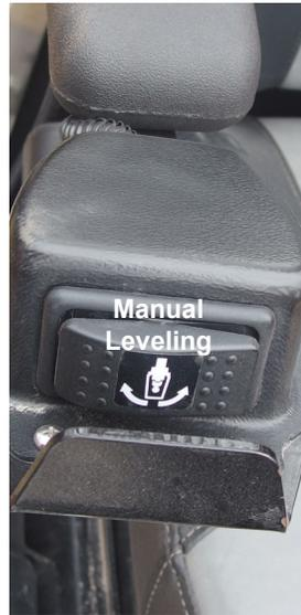
**Manual Leveling Switch** – one is located on the arm rest and the other on the ROPS. Both of these switches perform the same function. One is intended to be used while in the operator's seat and the other for when standing behind the machine. They are used to manually tilt the machine left or right.
