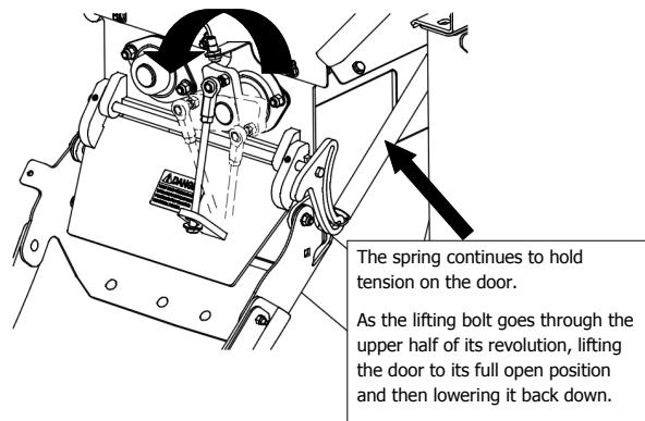
When it is in the closed position, it will create piles while operating. Where as if it is in the open position, it will create a row while operating.
