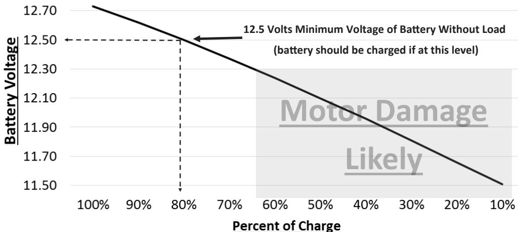
Chart Shows the unloaded voltage of a good battery at a particular charge level this is for reference only — actual battery charge and capacity should be determined by load testing of the battery
