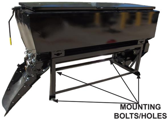
Put the Beefcake back in place where you marked and drilled the mounting holes. Attach with either the (4) mounting bolts included in your purchase or your own preferred size of mounting bolt that can fit into the predrilled mounting points on the Beefcake.
