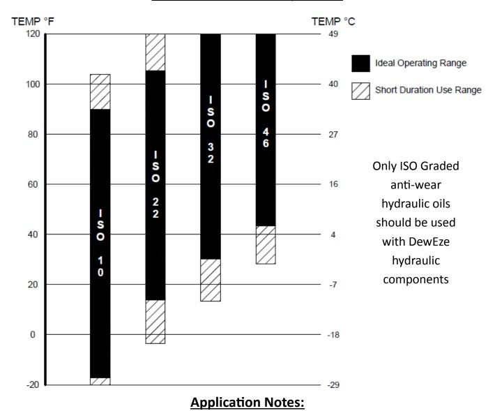
For Electric Drive Systems reduce by one viscosity grade due to reduced
