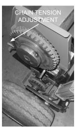
Check the condition of drive chain before each use or after every 25 hours of operation.
