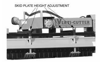
The skid plate height determines the cutting depth of the blades.
